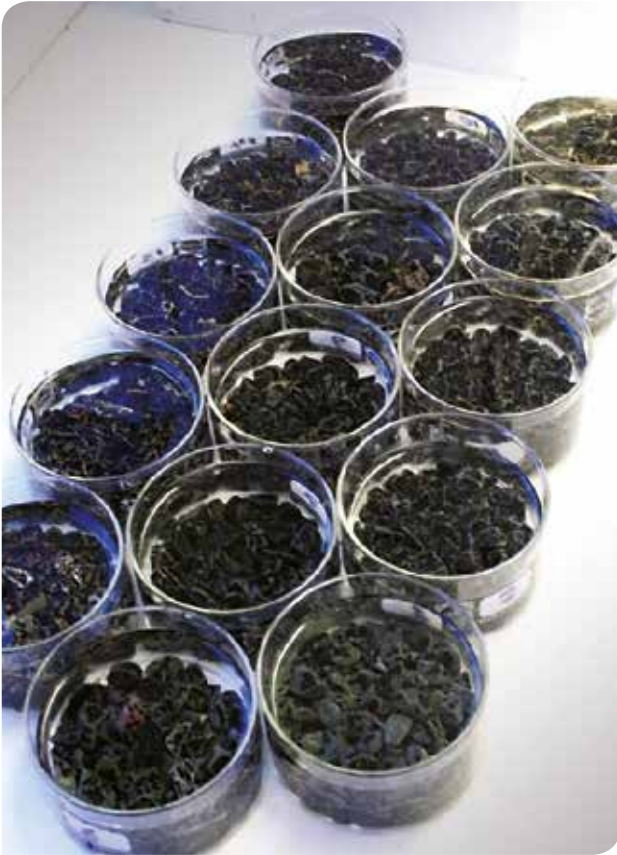
Static immersion test for surface dressing/chipseal.
