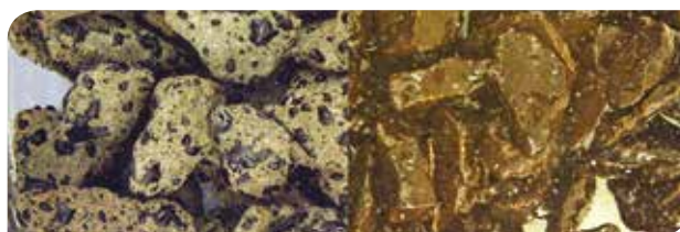
Static immersion test without adhesion promoter (left) and with Wetfix BE.
