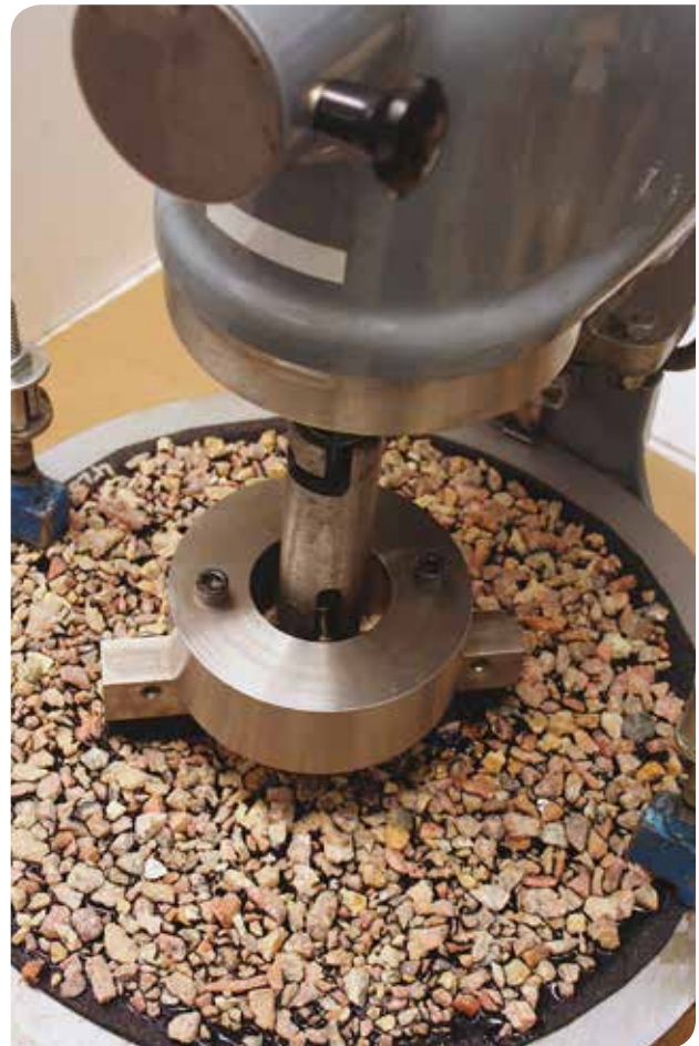
Surface dressing/chipseal sweep test.
