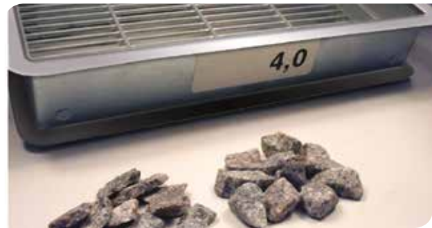
Measurement of Flakiness Index. Samples from the sieve test are passed through the slots.
